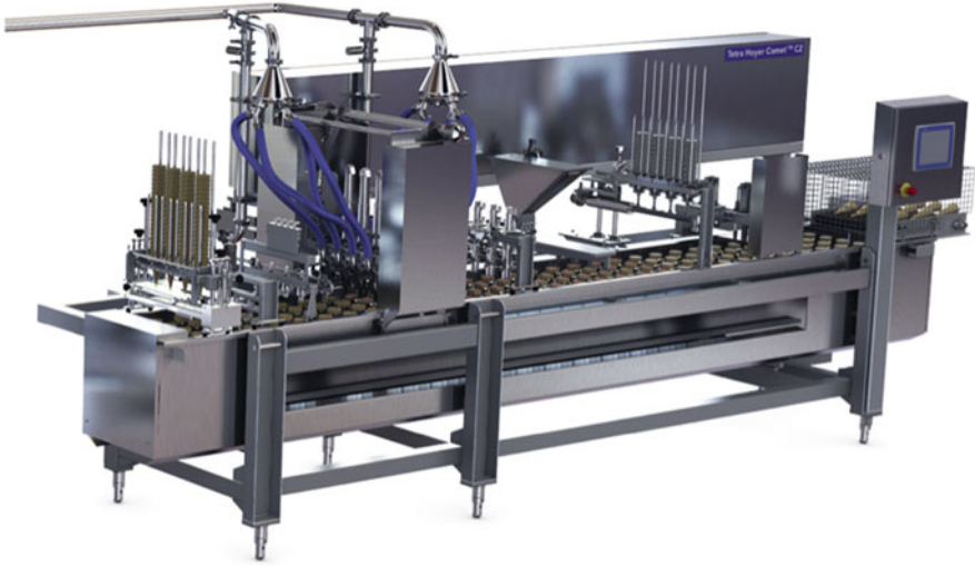
Fig. 10.7 In-line ice cream filler with multiple parallel lanes (courtesy of Tetra Pak Hoyer A/S, Højebjerg, DK)
