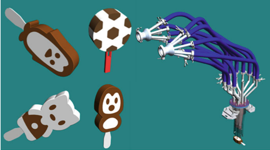
Fig. 9.17 Examples of the types of shapes and designs that are possible using vertical extrusion and an example of the filler head that would be required to direct differently colored ice creams to various parts of the design (courtesy of Gram Equipment of America, Tampa, FL, USA)
