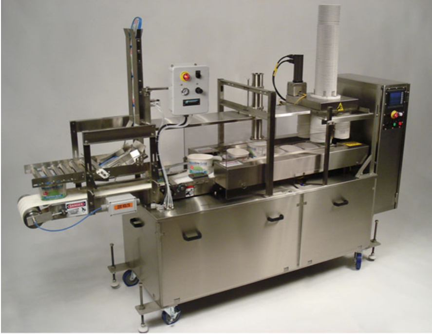
Fig. 10.5 In-line filler for square-round packages (courtesy of TD Sawvel Co., Inc., Maple Plain, MN)
