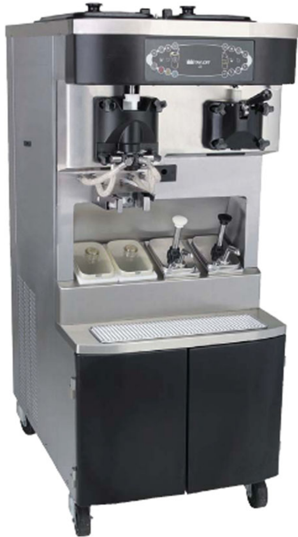
Fig. 8.3 A combination four-flavor milk shake/single-flavor soft-serve machine with four-compartment syrup rail for heated and room-temperature sundae toppings. This freezer also has heat treatment capabilities (Taylor Crown Series Model 606)
