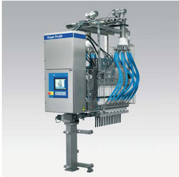
Fig. 9.10 Bottom-up filling machine for molded novelty machines (Hoyer Profill, courtesy of Tetra Pak Hoyer A/S, Højebjerg, DK)
