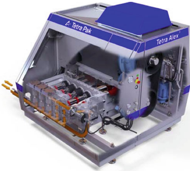
Fig. 5.10 Industrial five-piston homogenizer (TetraPak Alex), showing flow through the piston pump. The homogenizing valve assembly sits at the exit of the pump (courtesy of TetraPak Hoyer A/S, Høejobjerg, DK)
