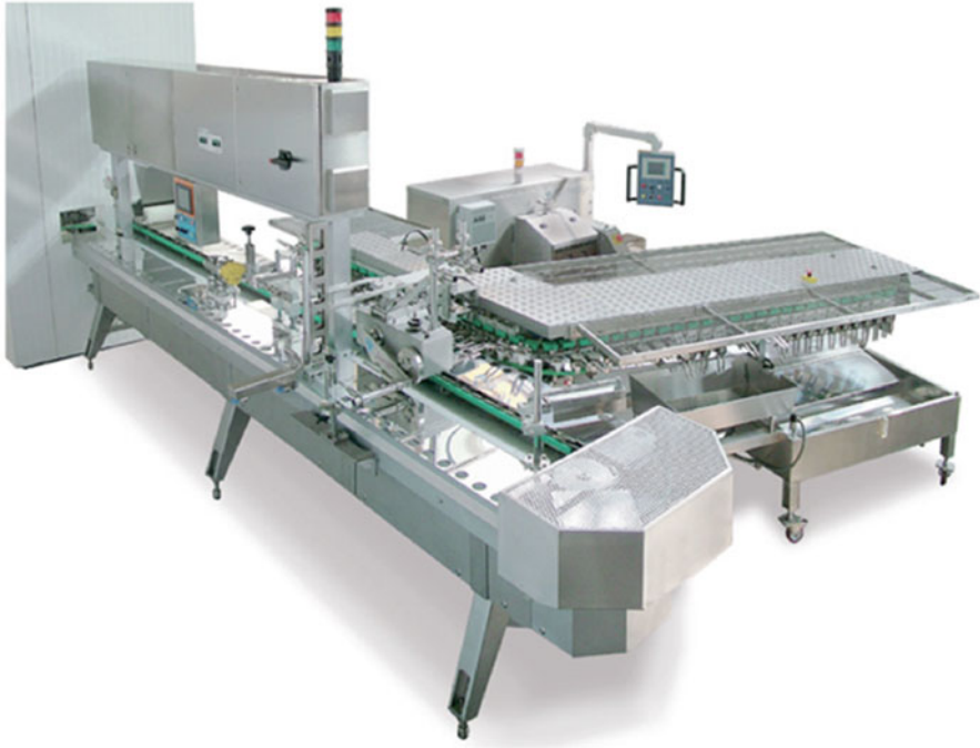
Fig. 9.15 Vertical extrusion machine for ice cream bars showing the filling side ( front ), plate conveyor system running clockwise to move product through the hardening tunnel (entrance to box tunnel shown at the left side), and product enrobing and wrapping lines after product exits from the hardening tunnel ( right side at the rear) (courtesy of Technogel, Bergamo, Italy)
