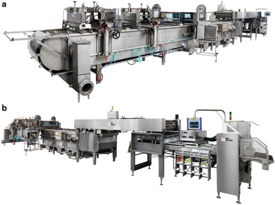
Fig. 9.7 Filling end (a) and extraction and wrapping end (b) of an in-line (straight-through) molded novelty machine (Versa-Line, courtesy of WCB Ice Cream, Northvale, NJ, USA)
