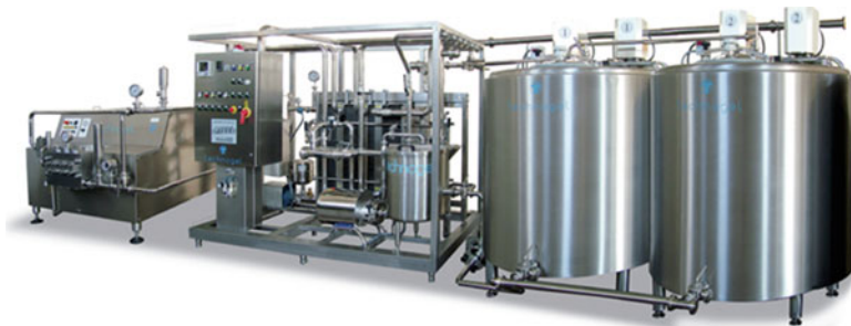
Fig. 5.9 Complete mix processing plant for small to mid-size operations, 600–5,000 L/h, including blending tanks, HTST pasteurization, homogenization, plate cooling, and aging tanks (courtesy of Technogel, Bergamo, Italy)
