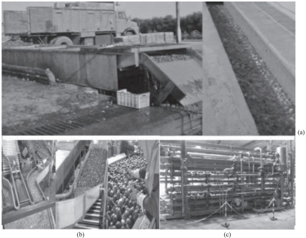
Figure 37.4 (a) Receiving and unloading tomato to soaking vat, (b) manual sorting, and (c) sterilization unit (Source: Rojin-Taak Agroindustry, Kermanshah, Iran).
