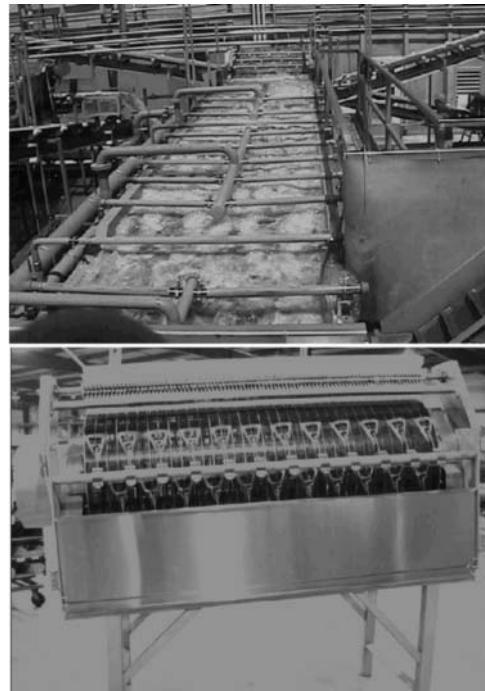
Figure 30.6 Green beans washing line (top) and stem snipper (bottom). (Courtesy: Lyco Manufacturing, Inc., Columbus, Wisconsin, USA.)
