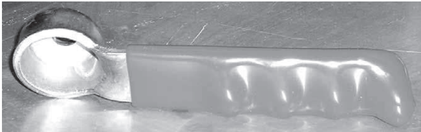
Figure 32: This simple crown capper is placed on the cap and hit with a hammer to bend the cap over the rim of the bottle.
